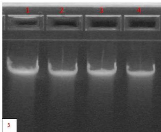
**Photo no 3:** results with NucleoSpin® Soil MACHEREY-NAGEL kit: 1 - sludge Line A; 2 - 0.25  $\mu$ m filter of 10 ml sample sludge Line A; 3 - sludge Line B; 4 - 0.25  $\mu$ m filter of 10 ml sample sludge Line B.
