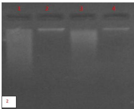
**Photo no 2:** results with DNeasy PowerSoil kit QUIAGEN: 1 - sludge Line A; 2 - 0.25 $\mu$ m filter of 10 ml sample sludge Line A; 3 - sludge Line B; 4 - 0.25  $\mu$ m filter of 10 ml sample sludge Line B.
